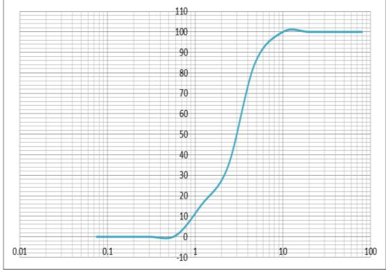
Figure 3: Particle size distribution curve for mill scale
