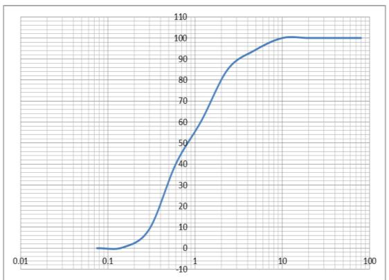
Figure 2: Particle size distribution curve for fine aggregate
