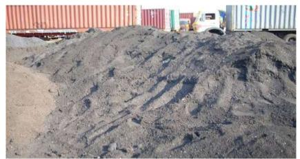
Figure 1. Steel mill scale
